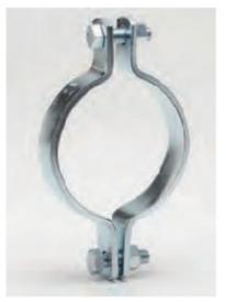
Pipe size: 1/8", 1/4", 3/8", 1/2", 3/4", 1", 1 1/4", 1 1/2" and so on. Thickness: 1.5mm, 2.0mm, 2.5mm, 3mm, 3.5mm. Design load: 1.8KN, 2.7KN, 3.6KN, 4.4KN. Material: carbon steel, copper, stainless steel. Finish: EG, HDG, Dacromet.
